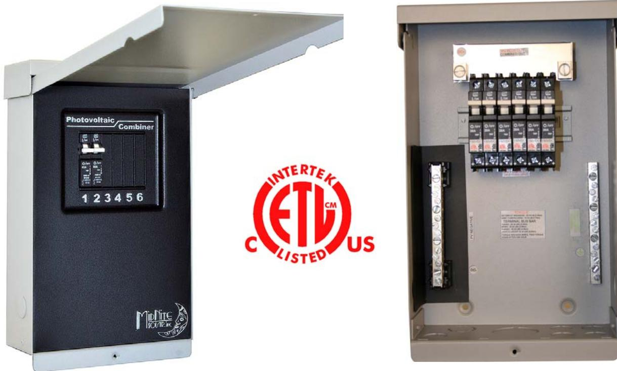
The MNPV6 combiner is rated for outdoor use. Designed for combining PV strings up to 150VDC and 120 amps total using breakers, or high voltage strings using 10mm x 38mm fuses up to 80 amps total. The use of touch safe din rail mount fuse holders and fuses allow operation up to 600 Volts. The MNPV6 combiner comes with two copper bus bars. One for circuit breakers and one for fuses. The MNPV3 busbar is designed for circuit breakers or fuses. The MNPV3 busbar is rated for 60 amps total.
