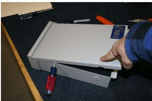
To remove the dead front: Pry off the lid as shown using something like a screwdriver as a lever. The dead front will then come out easily.
